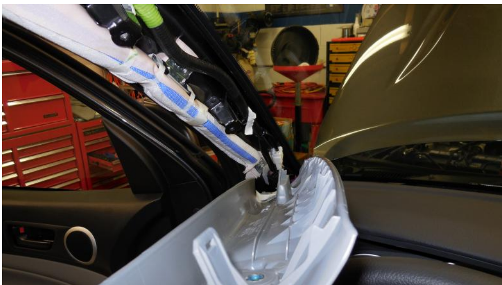
Remove the "A" pillar décor cover and put in a safe area.
