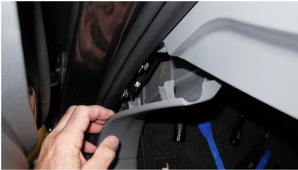
Remove the kick panel by pulling back.
