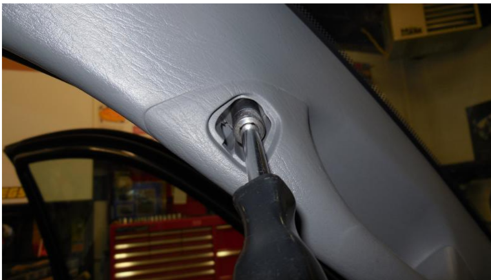
Using a Phillips screwdriver or 10mm hex socket (below) remove the hand grip.
