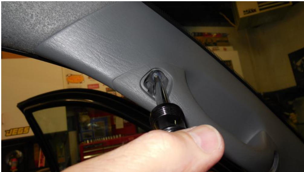
Using a Phillips screwdriver or 10mm hex socket (below) remove the hand grip.
